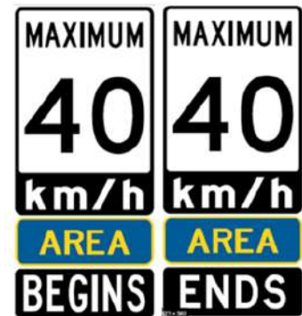
FIGURE 2.1: GATEWAY SPEED LIMIT SIGNS
